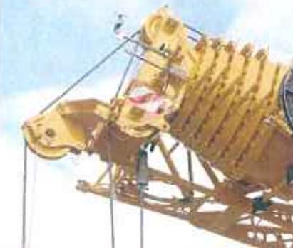
Hydraulic assembly assistance for attaching the folding jib
